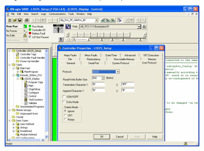
Load the application program and set the processor to "Run"
